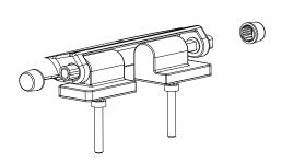
**Step 3** - Align and secure the adjustable buffers (8) into position. Ensure these are correctly fitted to position the seat centrally on the toilet.
