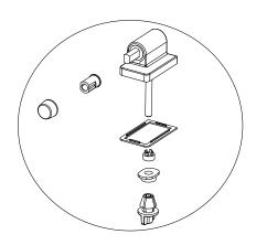
**Step 2** - Fit the hinge blocks to the seat. Note that the hinges are handed and must be fitted to the correct sides. Fit the Pivot caps (7) into place.
