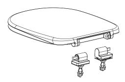
**Step 4** - Align the hinge blocks with the toilet holes and replace the spacer, washer and nut. Repeat for both sides and tighten into position. Ensure the hinge pad is correctly fitted.
