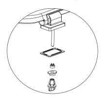
**Step 3** - Align and secure the adjustable buffers (8) into position. Ensure these are correctly fitted to position the seat centrally on the toilet.
