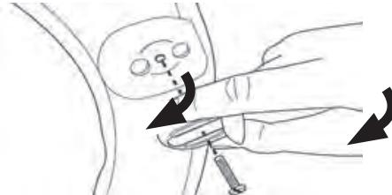
Fit the buffers with the tang to the inside. Insert the screw, FINGER TIGHT only.
