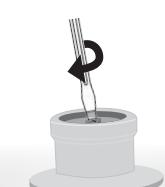
Remove the seat with the hinge pillars and tighten down the top fix bolts, using a suitable screwdriver.
