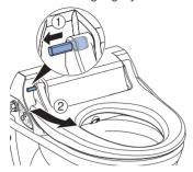
Pull the WC seat ring from the right hinge pin and remove it.
