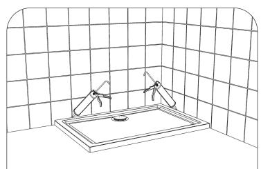
The tray should be tiled and grouted at this stage, seal the joints with a good quality bathroom sealant and allow to set.
