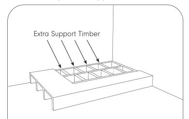
Cut extra lengths of timber to fit between the floor joists approximately every 250mm, this will provide additional support. Cut slots in the supporting timbers to allow the waste pipe work to run correctly.
