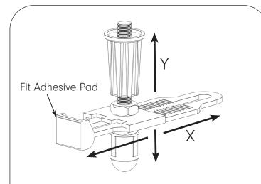
Fit the adhesive pads onto the front faces of the fascia to tray foot joints, leaving on the release paper till later on in the process.
