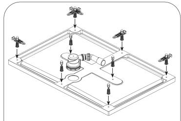
Screw in all the tray feet into the inserts on the underside of the tray until they bottom out, tighten the locking sleeve if the tray foot onto the tray. The feet should be set at 100mm from the underside of the tray to give a total height of 140mm (tray + feet).
