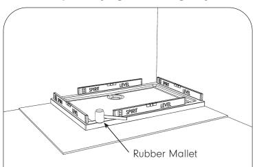
Fit the waste to the tray in accordance with the manufacturer's instructions, place the shower tray with the fitted waste onto the cement bed and gently tap the tray into position and then finally level the tray and allow to set.
