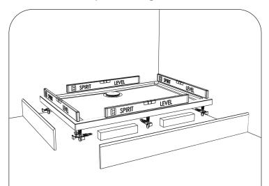
Cut the fascias to length to suit the tray. Measure the distance from the floor to the underside of the tray and carefully cut the fascias to these dimensions.
