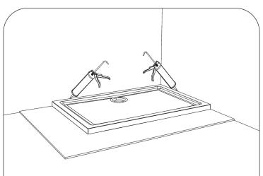
When the shower tray is set, connect the waste pipe and check all plumbing for leaks, flow and adequate drainage over the entire tray area.
