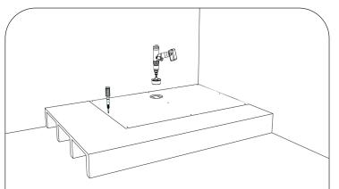
Prepare a rigid base of 9mm plywood where the tray will be positioned, incorporate a suitable recess or cut out for the waste. Screw-fix the plywood to the floor joists ensuring that the finished base is level and free from debris.
