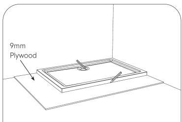
Prepare a rigid base of 9mm plywood, marking the perimeter of the tray and incorporate a suitable recess or cut out for the waste. Screw-fix the plywood to the floor ensuring that the finished base is level and free from debris.
