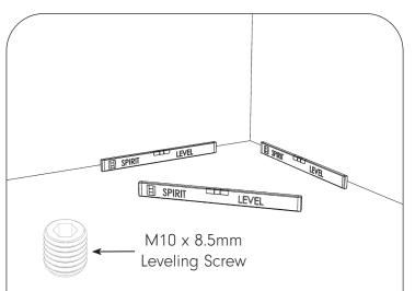
Prepare the floor on which the tray is to be fitted; ensure that there is adequate clearance for the waste assembly and outflow pipes. Caution should be taken to ensure there is adequate fall on the outflow pipe. High volume showers may require a greater fall.
