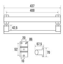
Elliptical tube in white epoxy-coated aluminium, 38 x 25 mm with wooden effect finish. Anthracite grey synthetic resin cover plates.
