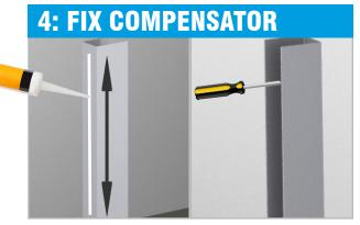
Run a bead of clear silicone bathroom sealant down the narrow face, for the full length of the outer compensator and then screw to the wall using suitable screws (**NOT SUPPLIED**). Wipe **ANY** excess silicone from compensator/wall joint.
