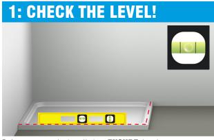
Before you start the installation, **ENSURE** that the shower area / shower tray / wetfloor former area where the doors are to fitted is level, from side to side and front to back, using a spirit level.
