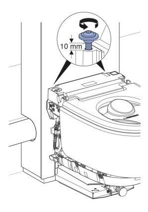
2 Assemble the standard side cladding parts.
