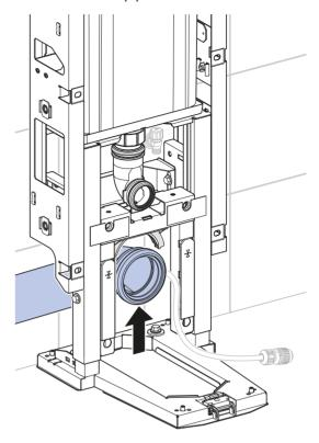
3 Secure the outlet pipe with the lower part of the pipe bracket.
