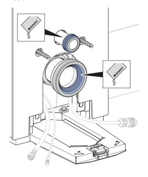
4 Mount the flush pipe and the outlet pipe.
