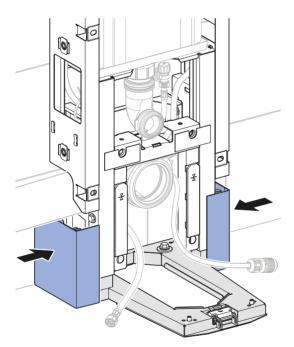
6 Lay the cables and the reinforced braided hose towards the front.
