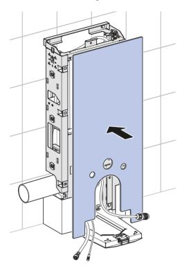
Press the front cladding into the frame to insert the interlock.
