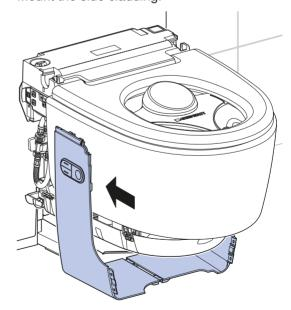
4 Screw the side cladding on securely.
