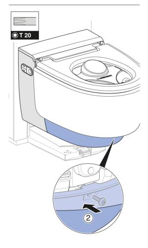
9 Mount the pedestal cladding for low or high positions.
