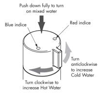
To turn on the mixer push down on the control knob until it contacts a stop and then release, mixed temperature water will flow for approximately 15 seconds.
