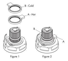
The thermostatic mixer tap has a factory set outlet temperature of 41°C via the security setting This is based on a balanced supply pressure and a stable hot water inlet temperature of 65°C.
