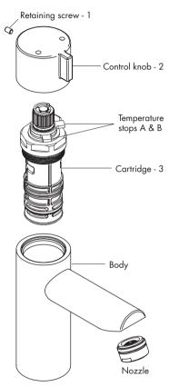
If the control knob cannot be depressed fully and does not return to its initial position within 15 seconds, or the temperature cannot be adjusted easily or water does not flow in a steady stream the mixer may require servicing.
