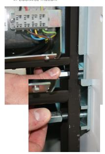
23 Loosen the counternut on the left support screw with an 8mm wrench in anticlockwise motion. Unscrew the support screw by hand until the mechanical stop. Re-tighten the counternut on the left support screw with an 8mm wrench in clockwise motion. Loosen the counternut on the right support screw with an 8mm wrench in anticlockwise motion. Unscrew the support screw by hand until the mechanical stop. Tighten the counternut on the right support screw with an 8mm wrench in clockwise motion.
