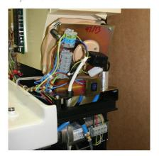
2 Allow approximately 5 minutes for the water to heat in the boiler. Check the circuit board, the boiler light will be permanently illuminated red while the water is being heated to the operating temperature. As the water temperature approaches the required operating temperature the light will flash red. If the boiler light does not illuminate, check the safety stat has not tripped (see inset) by pressing 'click' to reset.
