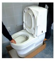
2 Remove the seat – Open the lid. Press and hold the seat pivots together with both thumbs whilst firmly gripping the outer edges of the seat. Now pull upwards sharply.
