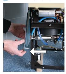
18 Attach assembly plate to the wall via the holes you have already drilled. Align the assembly plate horizontally with a spirit level. Tighten the four screws on the lift system with a 19mm wrench in clockwise motion. Remove the spirit level.
