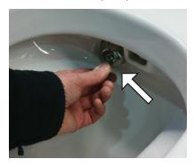
5 Pull out the douche arm using the special tool, with force against the spring pressure, until the arm reaches its maximum stop. Hold the douche arm with a free hand once fully extended, rotate the tool and locate the tool into the slot and recess in the douche arm to hold in this extended position (arrow). Run wash cycle to purge. Once wash is constant remove tool and allow the douche arm to retract.
