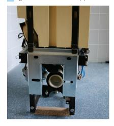
Loosen the nuts on the threaded pins of the mounting plates on both sides with a 13mm wrench in anticlockwise motion.
