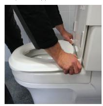
3 Carefully loosen and pull out the covering cap on the cistern cover.
