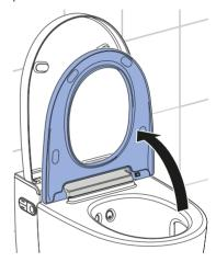
Slide the release button to the right and lift the WC seat ring out of the right-hand bracket.
