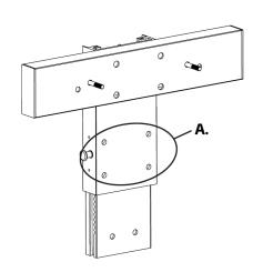
Adjust the lifting bracket in the highest position, tighten the adjustment screws visible in the four holes on the exterior profile. Run the lifting bracket up and down and make sure it runs smoothly.
