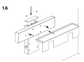
Install the cover plate and place the shelf as shown at the picture.
