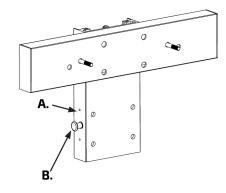
It is important that the sliding profiles are adjusted before you install the washbasin.
