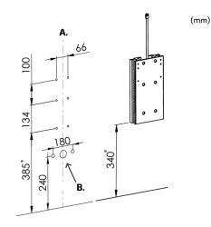
Water pipes are placed at c / c distance of 180 mm, 240 mm above the floor. Drains are placed between the pipes.
