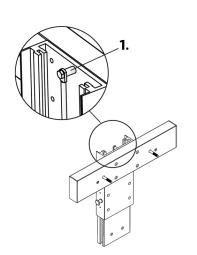
Lock the gas spring in the outer profile. The distance (1) shall be pinched between the gasspring and the outer profile. 1.4
