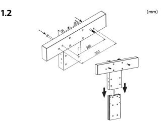
Push the bolts for washbasin. Place the bolts on the correct C / C distance for the basin to be used.
