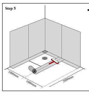
• From the wall mark out and apply joint tapes at 1000mm centres, overlap onto the floor/wall tape.
