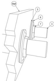
Looking at the wall from the front, the wall shrouds (4) may be screwed over the protruding unions (3) and fixed tight up to the wall.
