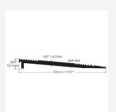
Interlocking aluminium grooved ramp, suitable for overcoming wheeled access issues. This ramp may be used on its own or with other sections from the RMP range to create different widths and heights of ramps. Rises from 0 to 12.7mm high x 100mm width. Gradient of 1:8. Aluminium, mill finish. Undrilled. Length (10ft) 3048mm.
