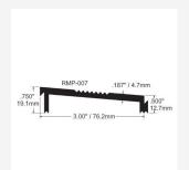
Interlocking aluminium grooved ramp section, suitable for overcoming wheeled access issues. This ramp can be used on its own as a bridge between existing floor surfaces and with RMP-001 for example to create a different width and length of ramp. Rises 6.4mm from 12.7 to 19.1mm x 76.2mm width. Gradient of 1:12. Aluminium, mill finish. Undrilled. Length (10ft) 3048mm.
