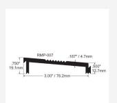
Interlocking aluminium grooved ramp section, suitable for overcoming wheeled access issues. This ramp can be used on its own as a bridge between existing floor surfaces and with RMP-001 for example to create a different width and length of ramp. Rises 6.4mm from 12.7 to 19.1mm x 76.2mm width. Gradient of 1:12. Aluminium, mill finish. Undrilled. Length (10ft) 3048mm.
