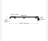
Interlocking aluminium grooved transition threshold that bridges from 12.7mm high on one side to 6.4mm high on the other, with a total width of 88.9mm. This threshold should be used with other sections from the AWS Modular Ramp System such as the RMP-001 for a 1:12 gradient or RMP-000 for a 1:8 gradient ramped threshold arrangement. Mill finish. Pre-drilled. Length (8ft) 3048mm.
