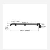
Interlocking aluminium grooved transition threshold that bridges from 12.7mm high on one side to 6.4mm high on the other, with a total width of 88.9mm. This threshold should be used with other sections from the AWS Modular Ramp System such as the RMP-001 for a 1:12 gradient or RMP-000 for a 1:8 gradient ramped threshold arrangement. Mill finish. Pre-drilled. Length (8ft) 3048mm.
