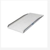
Standard Permaramp-original ramps are non-folding and without handrails. Semi-permanent and relocatable. Ideal for use with single outward opening doors with a timber or uPVC door threshold. Aluminium with the unique Gripdeck surface that offers an excellent all-weather grip surface while also being high heel and pet friendly. Width 76cm (30"). Length 210cm (7ft). Max. load 350kg (55kg). Ramp weight 22kg (49lbs).
