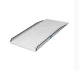
Standard Permaramp-original ramps are non-folding and without handrails. Semi-permanent and relocatable. Ideal for use with single outward opening doors with a timber or uPVC door threshold. Aluminium with the unique Gripdeck surface that offers an excellent all-weather grip surface while also being high heel and pet friendly. Width 76cm (30"). Length 240cm (8ft). Max. load 300kg (47kg). Ramp weight 25kg (55lbs).
