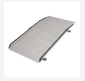
RampCentre Standard Utility ramp designed and manufactured for commercial uses with excellent load carrying capabilities. Width (excluding wheels) 76cm (30") x 210cm (7ft) length, with wheels on one side for easier movement. Manufactured from aluminium with the unique Grip deck surface that offers an excellent all-weather grip surface, retains grip even when wet. Weight 22.5kg (50lbs), maximum load 400kg (63st).
