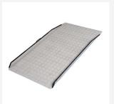
UR9 / (No Wheels) Standard, 76 W x 90cm L RampCentre Standard Utility ramp designed and manufactured for commercial uses with excellent load carrying capabilities. Width 76cm (30") x 90cm (3ft) length. Manufactured from aluminium with the unique Grip deck surface that offers an excellent all-weather grip surface, retains grip even when wet. Weight 9kg (20lbs), maximum load 400kg (63st).
