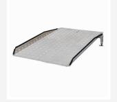
Standard Permaramp Adjust ramps are height adjustable between 7.5cm (3ins) to 25cm (10ins). A single length ramp that is non-folding and without handrails, they are semi-permanent and relocatable. The telescopic legs can be adjusted to accommodate timber and uPCV thresholds. The height can be adjusted from above. Width 76cm. Length 210cm. Max. load 350kg (55kg). Ramp weight 26kg (57lbs).
