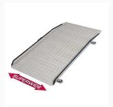
RampCentre Super wide Utility ramp designed and manufactured for commercial uses with excellent load carrying capabilities. Width (excluding wheels) 90cm (35.4") x 240cm (8ft) length, with wheels on one side for easier movement. Manufactured from aluminium with the unique Grip deck surface that offers an excellent all-weather grip surface, retains grip even when wet. Weight 30kg (66lbs), maximum load 300kg (47st).
