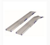
RampCentre Ultralight-Combi, unique lightweight channel ramps that are both folding and telescopic. Good for bridging door threshold with unequal levels each side and for bridging uPVC door thresholds. Overall length 210cm (6ft 11"), length of telescopic section 135cm (53"), length hinged section 75cm (30"), internal channel width 25cm (10"). Max. load (pair) 300kg (47st). Weight of each half 8kg (18lbs). Stored Dimensions L x W x D - 78 x 30.5 x 13cm (31 x 12 x 5"). Supplied as a pair.
