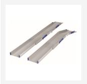
RampCentre Ultralight-Combi, unique lightweight channel ramps that are both folding and telescopic. Good for bridging door threshold with unequal levels each side and for bridging uPVC door thresholds. Overall length 300cm (9ft 10"), length of telescopic section 194cm (76"), length hinged section 106cm (42"), internal channel width 25cm (10"). Max. load (pair) 250kg (39st). Weight of each half 11.4kg (23lbs). Stored Dimensions L x W x D - 108 x 30.5 x 13cm (31 x 12 x 5"). Supplied as a pair.
