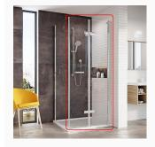
1967mm full height 800mm bi-folding doors with 755-775mm adjustment, part of a corner glass shower enclosure that also requires a fixed return panel to complete. Bright Silver coloured frame. 8mm thick glass. Unhanded - doors are reversible. Inward opening door with a 660mm aperture. Fits a shower tray with a front width of 800mm. Side fixed panel sizes available 760, 800, 900 and 1000mm. Glass pre-coated with Roman Ultra Care, a unique glass protection system. Made in the UK.
