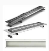
1000mm length Purus 100 stainless steel channel drain with a tile insert tray, ideal for shower areas, changing rooms, hotels, and leisure facilities with tiled floors. For installation in timber or concrete/screed floors. Heel-safe, suitable for bare-foot areas. End outlet with a choice of 3x plastic wastes, horizontal and vertical outlets. Or upgrade to the Acid proof stainless steel vertical 75mm outlet.
