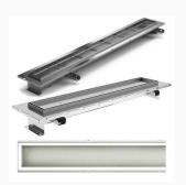
2500mm length Purus 100 stainless steel channel drain with a tile insert tray, ideal for shower areas, changing rooms, hotels, and leisure facilities with tiled floors. For installation in timber or concrete/screed floors. Heel-safe, suitable for bare-foot areas. End outlet with a choice of 3x plastic wastes, horizontal and vertical outlets. Or upgrade to the Acid proof stainless steel vertical 75mm outlet.
