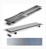
1000mm length Purus 100 stainless steel channel drain with a chess grid for tiled floors, ideal for shower areas, changing rooms, hotels, and leisure facilities with tiled floors. For installation in timber or concrete/screed floors. Heel-safe, suitable for bare-foot areas. Centre outlet with a choice of 3x plastic wastes, horizontal and vertical outlets. Or upgrade to the Acid proof stainless steel vertical 75mm outlet.
