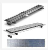
1200mm length Purus 100 stainless steel channel drain with a chess grid for tiled floors, ideal for shower areas, changing rooms, hotels, and leisure facilities with tiled floors. For installation in timber or concrete/screed floors. Heel-safe, suitable for bare-foot areas. Centre outlet with a choice of 3x plastic wastes, horizontal and vertical outlets. Or upgrade to the Acid proof stainless steel vertical 75mm outlet.
