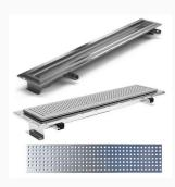
1000mm length Purus 100 stainless steel channel drain with a chess grid for tiled floors, ideal for shower areas, changing rooms, hotels, and leisure facilities with tiled floors. For installation in timber or concrete/screed floors. Heel-safe, suitable for bare-foot areas. End outlet with a choice of 3x plastic wastes, horizontal and vertical outlets. Or upgrade to the Acid proof stainless steel vertical 75mm outlet.
