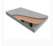
White 1800x900mm AKW Onyx shower tray leg kit, for corner or alcove installations and provides a solution for various bathroom types with unbreachable floors and uneven floors. The heavy-duty feet are height adjustable by 100-126mm, overall height of 144 - 170mm for full installation. Magnetic trimmable SMC skirting board (144mm cuttable up to 26mm). The kit includes an AKW GW90 Onyx gravity waste.
