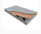
Grey 1400x800mm AKW Onyx shower tray leg kit, for corner or alcove installations and provides a solution for various bathroom types with unbreachable floors and uneven floors. The heavy-duty feet are height adjustable by 100-126mm, overall height of 144 - 170mm for full installation. Magnetic trimmable SMC skirting board (144mm cuttable up to 26mm). The kit includes an AKW GW90 Onyx gravity waste.
