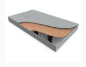
White 1200x800mm AKW Onyx shower tray leg kit, for corner or alcove installations and provides a solution for various bathroom types with unbreachable floors and uneven floors.The heavy-duty feet are height adjustable by 100-126mm, overall height of 144 - 170mm for full installation. Magnetic trimmable SMC skirting board (144mm cuttable up to 26mm). The kit includes an AKW GW90 Onyx gravity waste.
