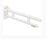
HEWI removable hinged support rail Duo Mobile, stylish powder coated matt white finish, two parallel round gripping levels made of high quality stainless steel. Maintenance free, permanently smooth and easy moving joint. With a 850mm projection, wall plate 210mm high and 101mm wide, loading capacity of 100kg. Toilet roll holder included.
