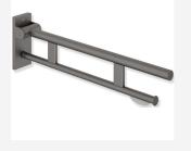
HEWI removable hinged support rail Duo Mobile, stylish powder coated matt dark grey pearl mica finish, two parallel round gripping levels made of high quality stainless steel. Maintenance free, permanently smooth and easy moving joint. With a 850mm projection, wall plate 210mm high and 101mm wide, loading capacity of 100kg. Toilet roll holder included.
