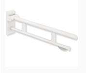
HEWI removable hinged support rail Duo Mobile, stylish powder coated matt white finish, two parallel round gripping levels made of high quality stainless steel. Maintenance free, permanently smooth and easy moving joint. With a 900mm projection, wall plate 210mm high and 101mm wide, loading capacity of 100kg. Toilet roll holder included.
