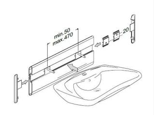
Bolt distance: Min. 50 - max. 470 mm.
