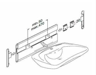
Bolt distance: Min. 50 - max. 470 mm.
