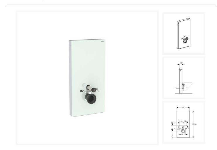
Geberit Monolith for wall-hung WC pans, installed height of 101 cm (1010mm). A stylish dual flush, selfsupporting concealed cistern that is fully insulated against condensation. The front panel is made of 6mm Mint glass with brushed aluminium side profiles.
