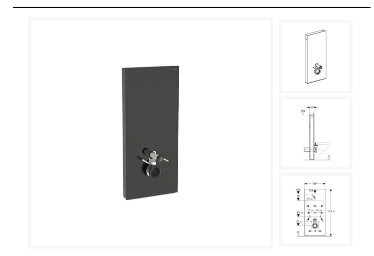
Geberit Monolith for wall-hung WC pans, installed height of 114 cm (1140mm). A stylish dual flush, selfsupporting concealed cistern that is fully insulated against condensation. The front panel is made of 8mm thick Black glass with Black Chrome brushed aluminium side profiles.
