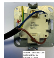
Baselift 6300 series control switch wiring Product Code: 61320
