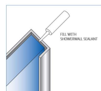
End trim 2450mm. Finishing end cap for square cut edge panel. Seal with Showerwall sealant.
