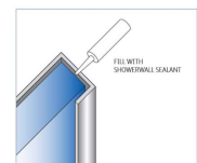
End trim 2450mm. Finishing end cap for square cut edge panel. Seal with Showerwall sealant.
