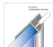
Quadrant trims 2450mm. Finishing end cap for square cut edge panel. Seal with Showerwall sealant.
